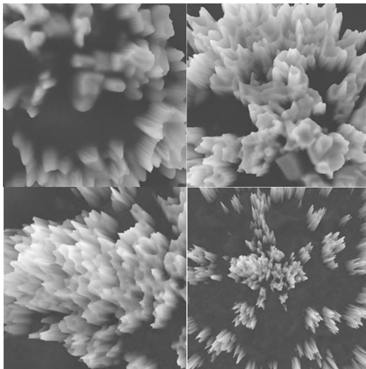
Fig. 5. SEM (3D) image of ZnO nanopowder 41nm at different magnifications.
