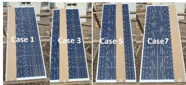
Figure 13. Shading positioning on the PV module.
