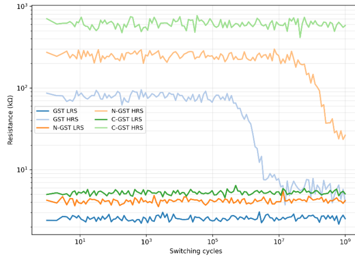
Figure 7. Endurance performance. Evolution of R_{HRS} and R_{LRS} for GST, N-GST, and C-GST devices over repeated switching cycles.
